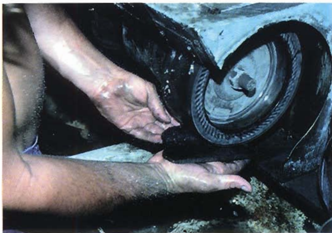
Jeff Kline puts it through the paces. Saw marks must be polished out through at least 220 grit to properly prepare an iron meteorite for the etching process.
